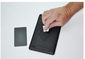
8. Remove the protective backing from the tablet adapter. Find the center of the tablet, then line up the adapter so that is evenly spaced. Place one edge of the adapter against the tablet as shown. Once you have confirmed the adapter is centered, rest the adapter against the tablet and press into place.
