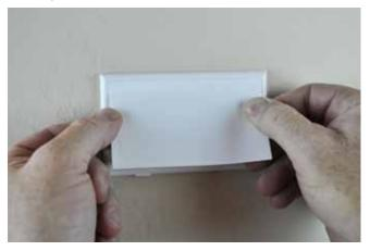
8. Remove the remaining backing from the rubber face. Carefully attach the remaining face rubber, lining it up with the edges as you work your way across. Be sure to press out air bubbles as you attach the rubber.
