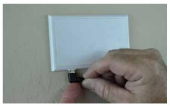
12. Plug the other end of the wire into your tablet. Then, attach the tablet to the S-Mount-POE. Route any extra wire behind the tablet so that it is hidden from sight.
