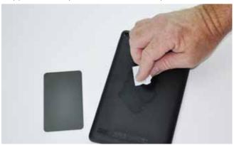
10.Remove the protective backing from the tablet adapter. Find the center of the tablet, then line up the adapter so that is evenly spaced. Place one edge of the adapter against the tablet as shown. Once you have confirmed the adapter is centered, rest the adapter against the tablet and press into place.
