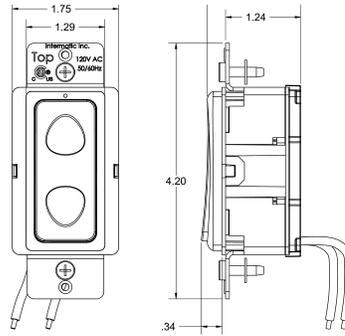
The CA5100 Accessory Wall Switch Controller is a Z-Wave™ enabled device which is fully compatible with any Z-Wave enabled network. Z-Wave enabled devices display the Z-Wave logo and guarantee connectivity and interoperability between devices. Each line powered node in a Z-Wave network is designed to act as a repeater forming a mesh network eliminating radio “dead spots” and providing the highest level of reliability.
